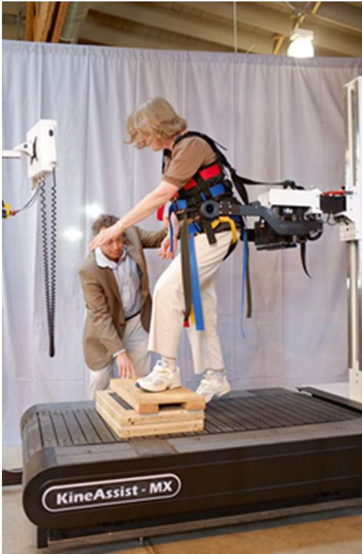
**Fig. 3.7** Example of robotic device (KineAssist MX, HDT Robotics) that was used to enable to stroke survivors to practice highly challenging balance and walking tasks while also providing safety and stability against falls. (Photo courtesy of HDT Robotics)
